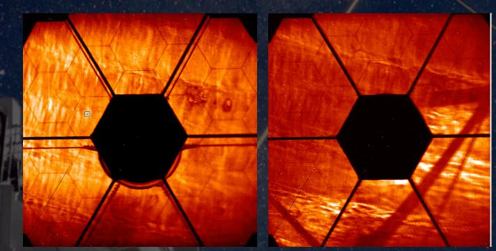
Telescope pupil image before and after alignment with NIRC2 "largehex" mask
